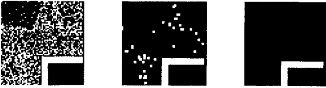
Figure 8: A noisy image and the results after applying morphological opening filter.
