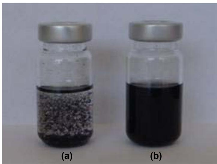
**Fig. 2** Vials containing CN<sub>x</sub> tubes grafted with polystyrene (PS). There are clear differences in organic solvents (i.e. toluene) between **(a)** physical blend of PS and CN<sub>x</sub> tubes, and **(b)** PS-CN<sub>x</sub> tubes polymerized in-situ.
