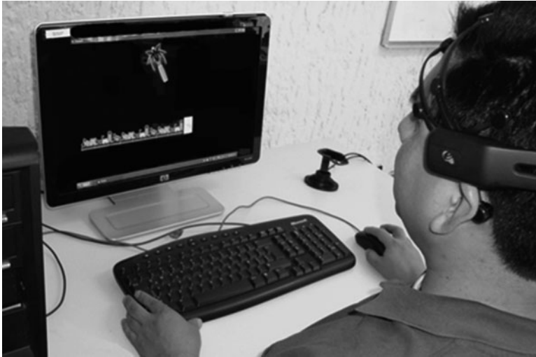
Fig. 27.3 Headset and stimulus used for the experiment on P300 signal detection
