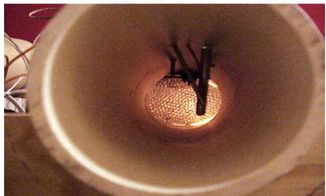
Fig. 2. Cross section of the inner pipe showing the sensors, gauge and bulb.
