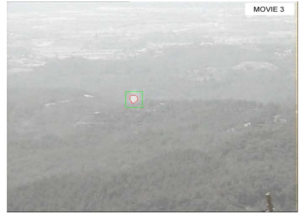
Figure 5. Sample image from movie 3 successfully detecting smoke
